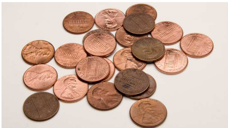
The shiny parts of these pennies are from the copper atoms that make up the pennies. The dull parts are from copper oxide, which forms on the surface of pennies over time.
