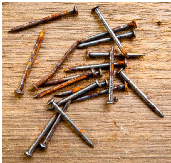
These nails are in various stages of rusting.
